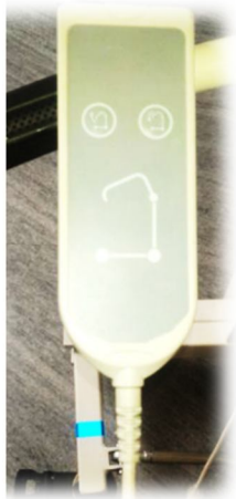
REMOTE & BATTERY BOX WITH INDICATOR & EMERGENCY STOP BUTTON MOUNTED TO BACK OF THE DEVICE.
