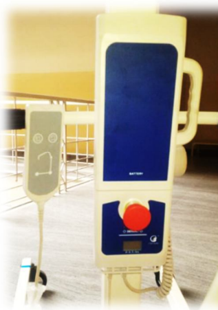
REMOTE & BATTERY BOX WITH INDICATOR & EMERGENCY STOP BUTTON MOUNTED TO BACK OF THE DEVICE.
